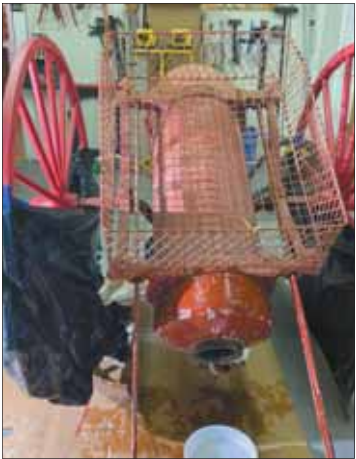
This fire cart was in service in Homedale in the early 20 th century. According to information planned for the Owyhee County Historical Museum exhibit, the cart carried two chemicals and was stored upright. A cylinder was screwed down on top of the cart when deployment was necessary, and when the cart was tipped onto its wheel, the chemicals mixed to produce a pressurized fire retardant.
